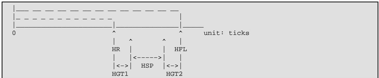
Now, we would like to place a sync pulse of length HSP as shown above, ie, between the end of clock ticks for display data and the end of clock ticks for the entire frame. Why so? because if we can achieve this, then your screen image won't shift to the right or to the left. It will be where it supposed to be on the screen, covering squarely the monitor's viewable area.
