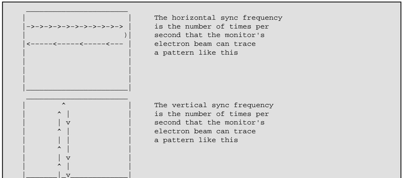
Remember that the actual raster scan is a very tight zigzag pattern; that is, the beam moves left-right and at the same time up-down.
