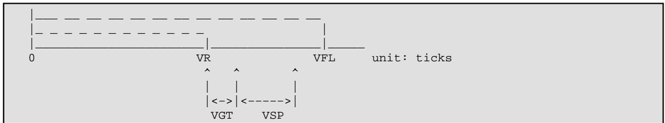
We start the sync pulse just past the end of the vertical display data ticks. VGT is the vertical guard time required for the sync pulse. Most monitors are comfortable with a VGT of 0 (no guard time) and we'll use that in this example. A few need two or three ticks of guard time, and it usually doesn't hurt to add that.
